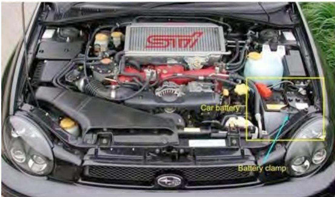
Batteries can be located in the engine compartment, under the drivers foot well, in the wheel arch and in the boot, these are the most common places to look however they may be in other locations.
