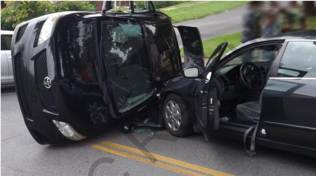
Vehicle relocation can be used for any situation, it has historically been used to move a vehicle resting on its wheels to provide access to a secondary vehicle, usually with no casualties in the vehicle being moved. We are comfortable with this mostly because there aren't any casualties in the relocated vehicle. Which I would agree is a common thought.
