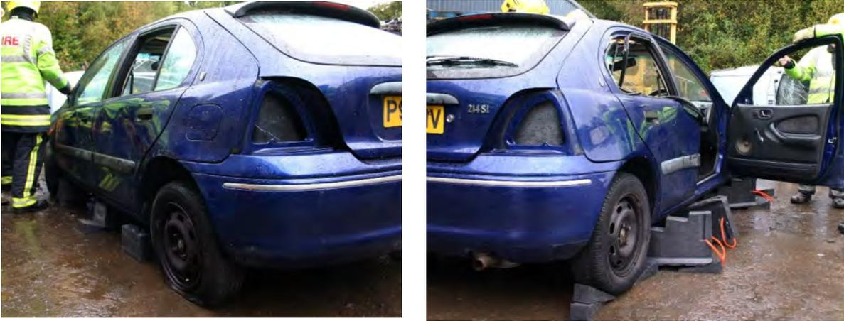
You can see in the above pictures the difference between the two types of equipment used with regards to trip hazards etc. Both sides stabilised ready for a dash roll. You can see on the right picture that there is also a risk that the rear door may come into contact with the rear step block, it would perhaps have been better placed at an angle, and this picture is just for training purposes.
