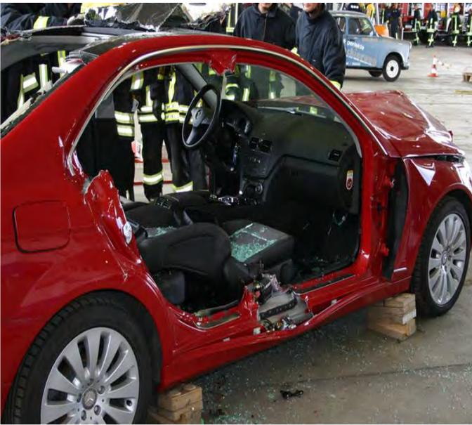
These cuts were carried out on new cars with UHSS components, as you can see ripping the B-post was successful.
