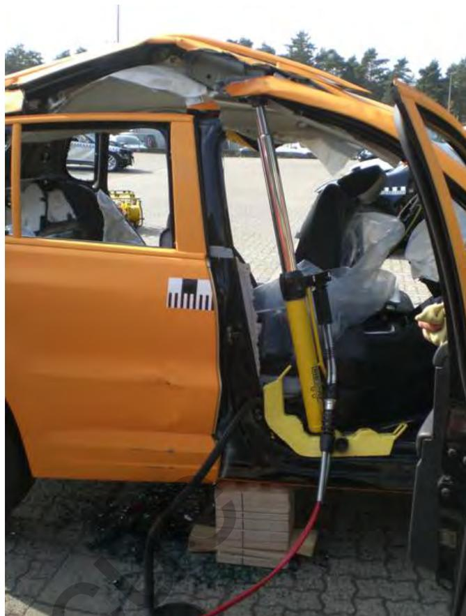
In the old days and for some this may still be the case, when we only had Combi tools on our trucks we always carried out a B-post rip as this was easier than trying to cut the post off, but as we progressed with dedicated cutters we now tend to primarily cut the B-post off at the base.
