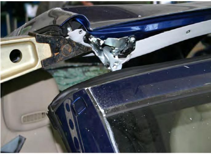
Another method is the tent technique, which does not create maximum space, but where we are unable to cut the roof posts we can give ourselves that bit extra space to work with.
