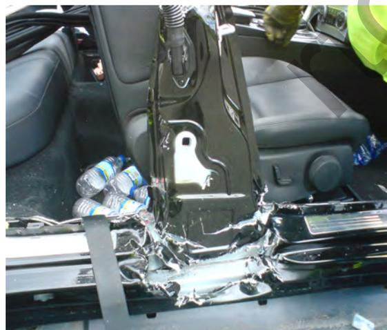
On the left you can see a Brand new Mercedes we were unable to cut the base of the B-post, even after trying as you can see it remained solid.
