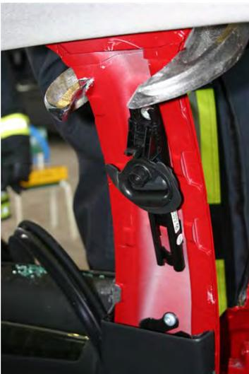
If you are dealing with a Coupe or a Convertible, expect that there are UHSS pipes in A-post and probably the remains of the B-post (Coupé). Try to avoid cutting those pipes, therefore, cut high on the A-post of a convertible or do something else to remove the roof. Some of the pipes cannot be cut, even with late model cutters, especially when mounted deep inside the pillar.
